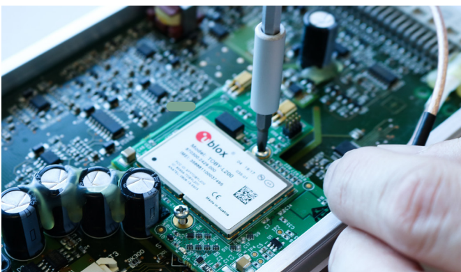
NW-4G LTE modem board installation
