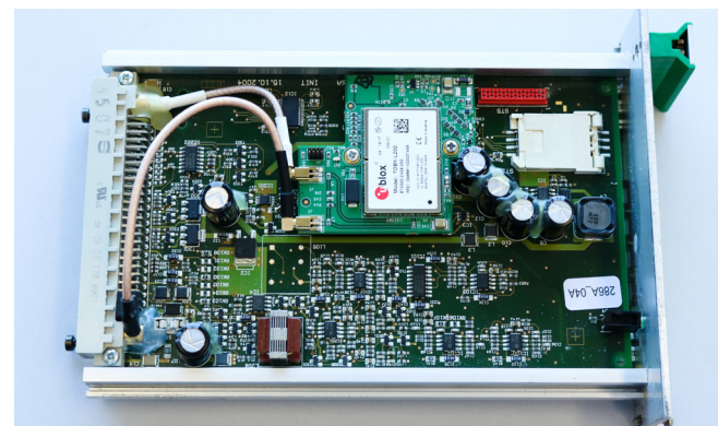
NW-4G LTE modem board installed in INIT transportation system
